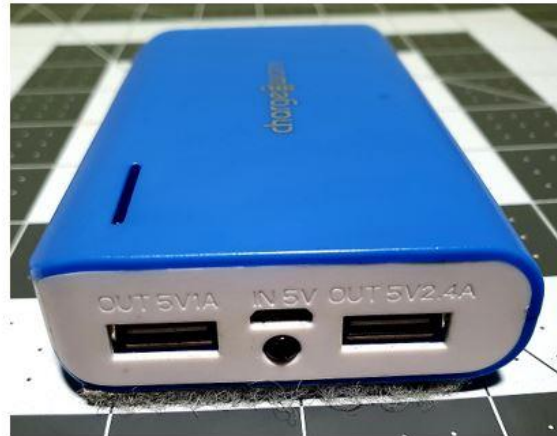
Portable battery charger (6000 mAh 3.7V, Out 5V, Output Max. 2.4A)
